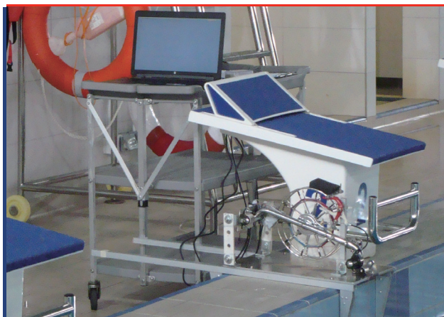
Figure 1. Cable tethering speed-time monitoring device setup
